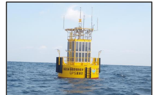
GPS buoy measures water level Source: Ministry of Land, Infrastructure , Transport and Tourism
