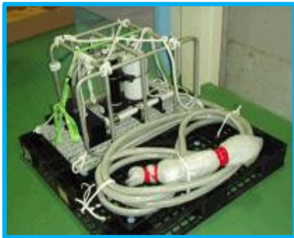
Pressure Gauge measures water Pressure
