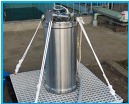
Seismometer measures acceleration
