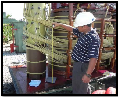
Locate fault based on AE location
