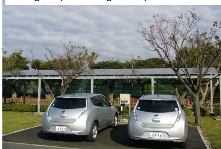
Charged by PV during the daytime at CRIEPI
