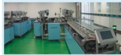
Measurement and test equipment: Automatic verification system with low voltage current transformer
