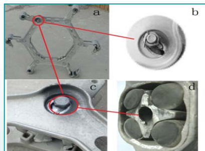
Wind damage on spacers
