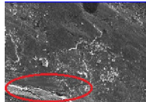
Abrasive wear microanalysis
