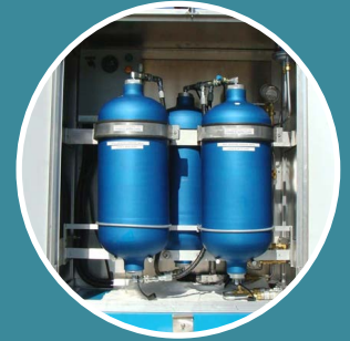
Corrosive Sulfur & PCB Removal Unit
