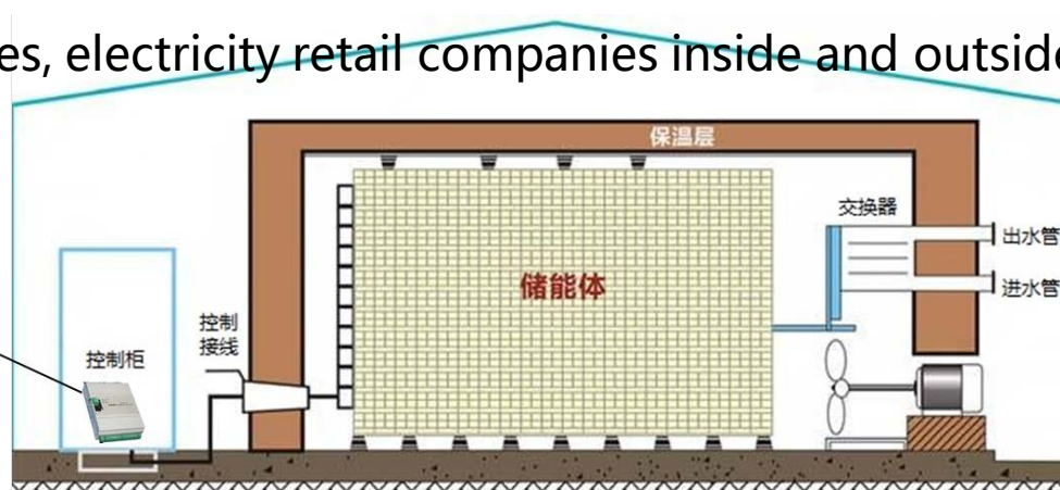
Application schematic diagram of interactive module for electric heat storage boiler-oriented demand response
